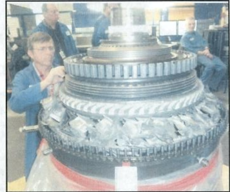
AVP-100's Bob Hendrickson examines the damage to the first stage of the high pressure turbine section of a GE GenEx engine from a foreign carrier.
